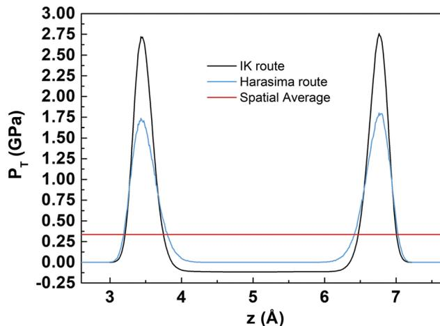
Fig. 1 Local tangential pressures using the IK and H definitions, and the spatially averaged tangential pressures (eqn (2)) for four different definitions of  $C_{ij}$  (the IK and H definitions, and two alternative contours), for LJ argon in a slit carbon pore of width  $H = 3\sigma$  at 87.3 K, 1 bar bulk pressure.<sup>15</sup>
