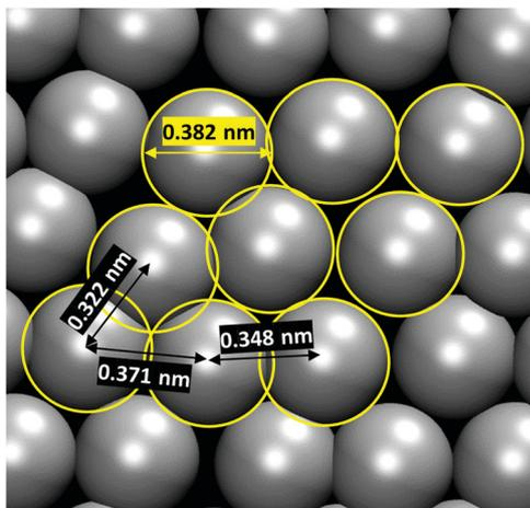
Fig. 2 An in-plane view of the contact layer next to the carbon wall for LJ argon in a carbon slit pore of width  $H = 3\sigma$  at 87.3 bar, 1 bar bulk pressure, showing separation distances between neighbouring molecules. The open circles show the nearest neighbor separation, 0.382 nm, when there is no compression, *i.e.* the intermolecular force is zero. Overlap of open circles implies strong repulsion between neighbouring pairs (see Fig. 4 of ref. 1 and 17).
